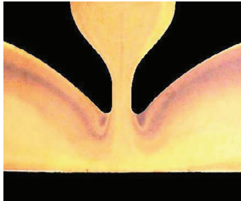
Fig. 7. Experiment: flow visualization at Re = 356 shows only vestigial patterns at the nozzle lips caused by the strong direction changes ("bends") on both sides of the jet - but no "dominant vortices".
